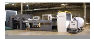
The MAXSON MSU Sheeter delivers up to 18,000 press ready sheets per hour to the printing press feeder without increasing the size of the operating crew.
