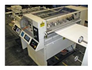
The MAXSON MSE Sheeter can be outfitted with a slitter rig for multiple pile service and/or electronic drives for press ready accuracy
