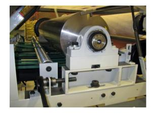
With a maximum speed of 300 fpm (90 mpm) the MSE Sheeter can convert up to 1 ton (910 kg) of board an hour.
