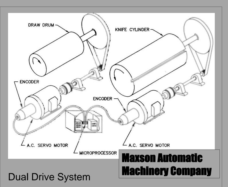
This stationary bed knife sheeter retrofit package replaces a cutter's existing wear-prone mechanical transmission or obsolete electronics with a reliable electrical system. The drive system allows cutoff lengths to be set in seconds, assures accuracy levels, and reduces maintenance levels of drive components. The sheeter's electrical system is comprised of drives and programmable controller in a UL approved electrical enclosure, motors and Operator interfaces.
