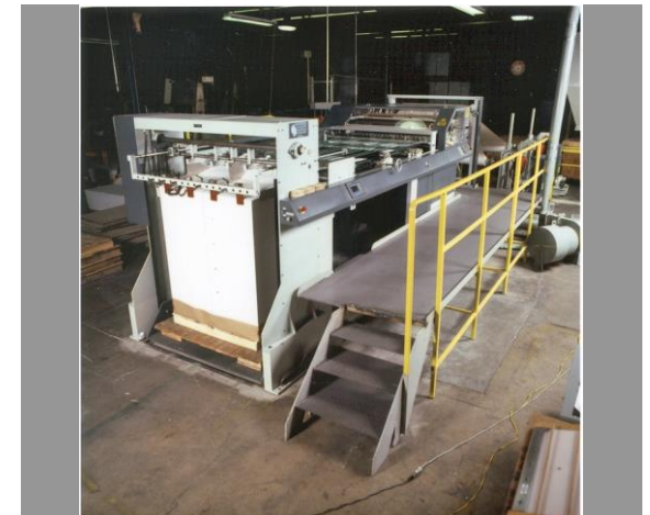
MAXSON MSP Sheeter with Series 200 Stacker, designed for the digital press size market.
