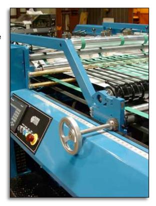
Connecting frames on either side of the overlap carriage are attached to the stacker's front stop assembly, which is positioned to allow sheets to be tightly jogged into a well formed pile. By moving the overlap carriage, the front stop assembly is automatically set, eliminating the need for the Operator to walk from the delivery system to the front of the stacker and properly set up the stacker.
