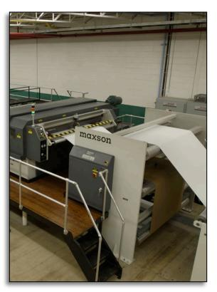
drives are governed by a microprocessor enabling size changeovers in less than two minutes. Outfitted with digital electronic controls, accuracies within + 0.010" (+ 0.254 mm), are maintained. Because the speed of the blades match the speed of the web at time of cut, no adjustment for squareness is required.
