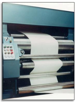
adjusted by varying the air pressure fed to the dancer roll cylinder.
